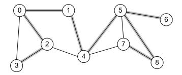
Figure 3: A Graph and A Spanning Tree
