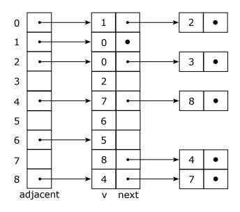
Figure 5: An Adjacency Lists Representation of a Graph
